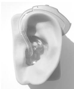
To remove ear mould, pull ear back slightly and slot thumb or finger under the mould. Flick the mould out. Once out disconnect the battery by opening the battery drawer.
