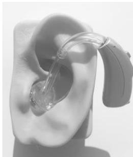
Place the hearing aid over the back of your ear. If the battery drawer was open then now close it to turn the hearing aid on.
