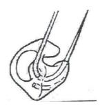
4. Cut off the tapered end as close to the mould as possible.
