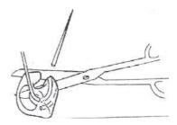
To adjust the tubing to the right length, place the mould in your ear and the hearing aid over the top of your ear. Ask somebody to make a mark where the tubing and end of the hook / elbow meet.
