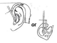
Cut the tubing at this point. Another method is to hold the old piece of tubing against the new piece of tubing and cut it to the same length.
