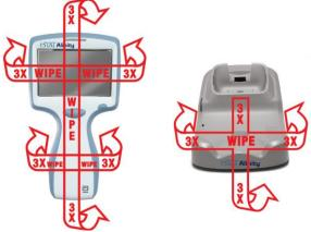
Clean the docking station and Electronic Simulator when/if required.
